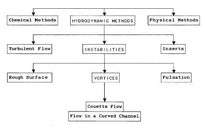
FIG. 1 Typical methods to reduce concentration polarization and membrane fouling
